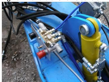
Fig.26 – Hand brake valve control
