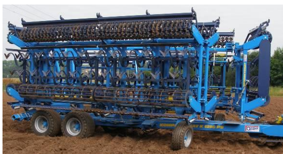
Fig. 30 – Transport position for ploughshare section replacement
