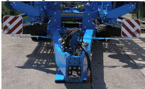
Fig.17 – Placing the front safety shields
