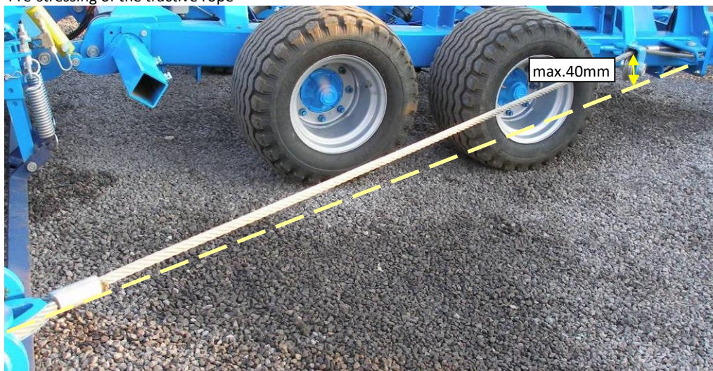
Fig.24 – Pre-stressing of the tractive rope
