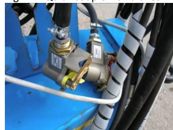
Fig.27 – Quick coupler for brakes
