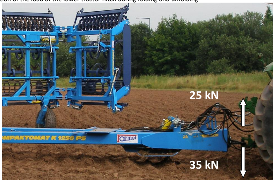
Fig.6 –Illustration of the load of the lower tractor hitch during folding and unfolding
