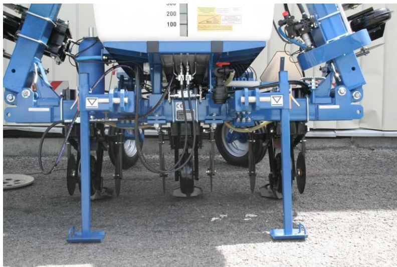
Fig. 2 Supporting Legs of the Machine in the Storage Position
