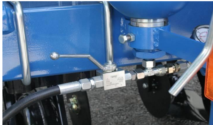
Fig. 6 Hydraulic Pressure Valve in Open Position
