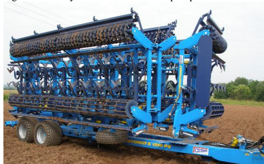
Fig.9 – Auxiliary wheels are in the transport position
