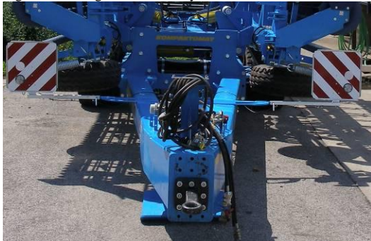
Fig.17 – Placing the front safety shields
