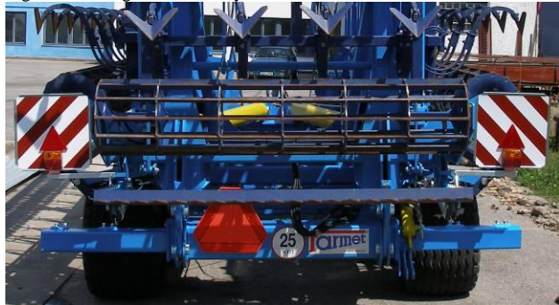
Fig.18 – Placing the rear safety shields
