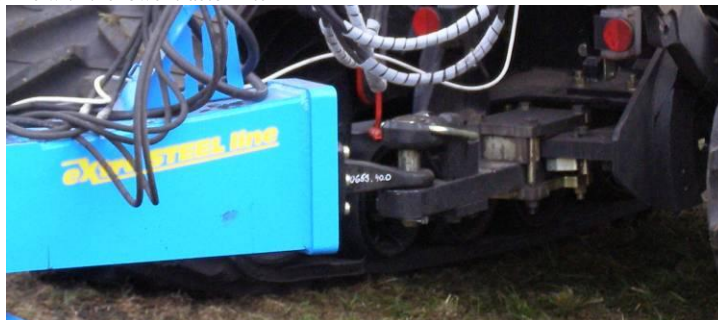
Fig. 5 – Connecting the machine with the lower tractor hitch
