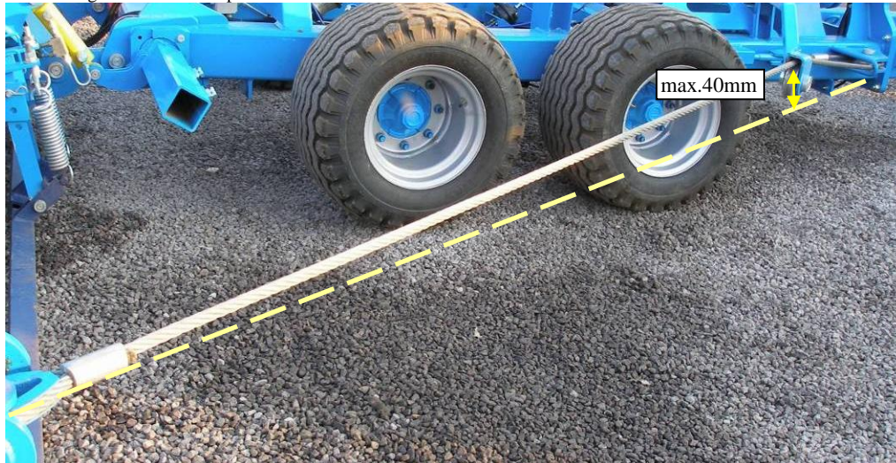
Fig.24 – Prestressing of the tractive rope
