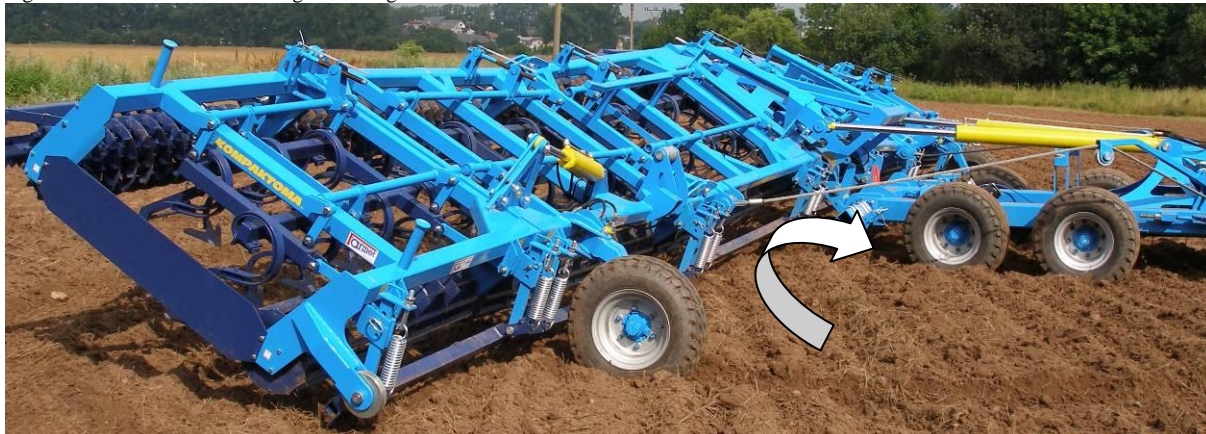
Fig.15 – Closing the working sections into the transport position
