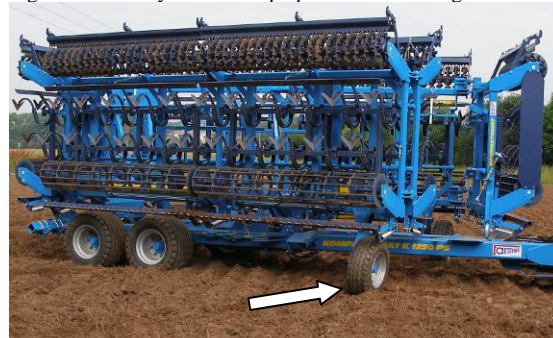
Fig.10 – Auxiliary wheels are prepared for unfolding
