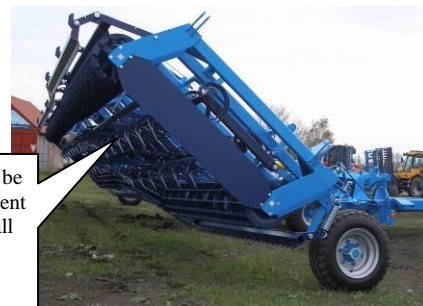
Fig.31 – Working section for ploughshare replacement in the field
